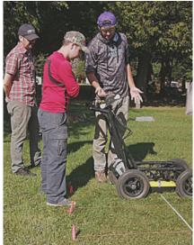
or ground penetrating radar. It is a device, which scans the subsurface of a gridded area using radar pulses to detect objects which lie beneath the surface. The result is a mapping of the area noting anomalies, natural obstructions and producing updated georeferenced drawings.
